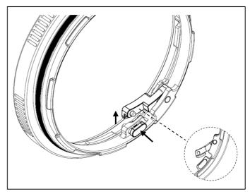
Push the blue released button and confirm that the extension ring is unlocked, with the locking lever upwards as shown.
