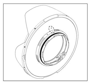
Align the "I" mark on the extension ring with the WHITE dot on the port.
