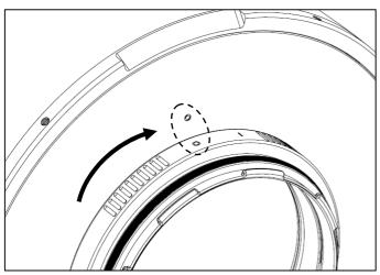
Turn the extension ring clockwise until the "O" mark on the extension ring aligns with the white dot on the port.
