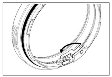
To lock the extension ring, push the locking lever downwards.
